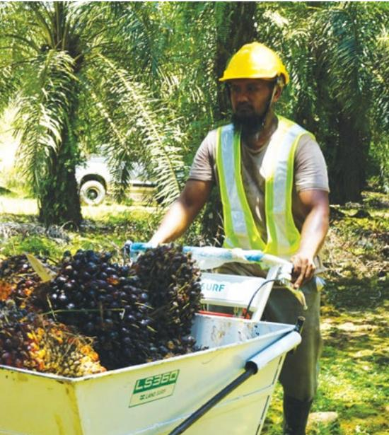
To further enhance operational efficiency in view of the reduction in manpower, Ladang Cendana is utilising the Land Surf, which is a motorised wheelbarrow, for collecting and evacuating FFB from the fields to the collecting point. This method has significantly improved the harvesters' productivity throughout FYE2023.
